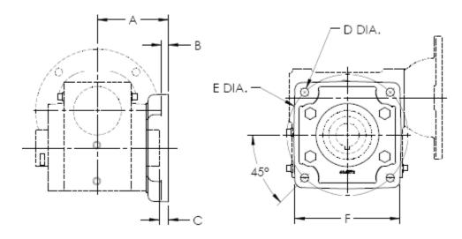
Output flange may also be used on solid output shaft reducers.
