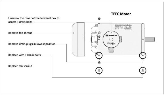
Figure 2 T-drain bolts
