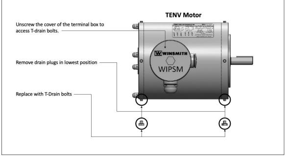
Figure 1 TENV T-drain bolts
