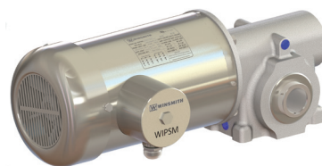
MPMS/TEFC Stainless Hollow Bore Output Shaft with Set-Screw Connection Totally Enclosed Fan Cooled Gearmotor (TEFC)
